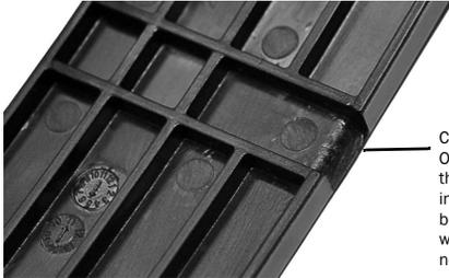
CLOSE-UP VIEW OF THE BACK OF THE FRONT PANEL - Note that there is a notched area in the exact center of the bottom. To remove, you must wedge a screwdriver into this notched area.
