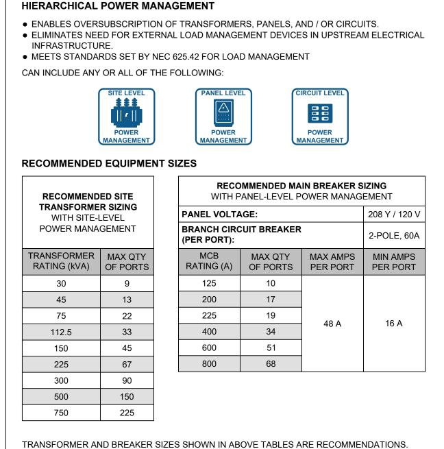
E.E. AND/OR E.C. TO VERIFY ELECTRICAL SPECIFICATIONS MEET CODE REQUIREMENTS. RECOMMENDATIONS ABOVE MAINTAIN A MINIMUM OUTPUT OF > 3.3 kW PER PORT @ 208 V~.
