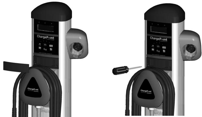
2. Using a T25 Torx driver, loosen the two captive security screws located at the bottom of the head assembly
