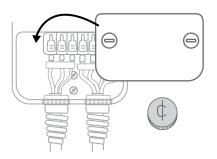
**Tip:** To avoid damage, do not use a screwdriver
