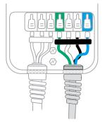
**Tip:** The cable clip protects the cord from damage
