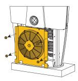
**5** Release the two cooling hoses located behind the fan by pulling the quick release sleeve. A drop or two of coolant may come out when the connectors are uncoupled. This is normal.
