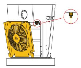
Remove the fan by unfastening its four nuts using an 8mm (5/16") nut driver. Slide the fan off the fasteners and place it on the base plate. Store the fasteners in safe place. Gently pull the fan about 2" forward taking care to avoid pulling on the fan wires or coolant hoses.
